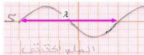
$$v = \lambda \times \nu = 5 \times 10^{-2} \text{ m} \times 100 \text{ Hz} = 5 \text{ m/s}$$
